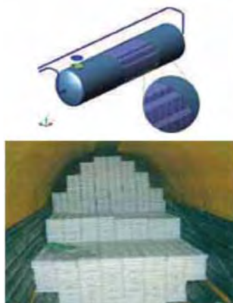
The FlatICE containers are designed to stack on top of each other forming a self-assembling heat exchanger within the tank above and top right). The Jeddah station project will utilize a 2.5 meter by 8 meter pressurized tank, like the one illustrated above left, that will house 5,500 FlatICE containers.
